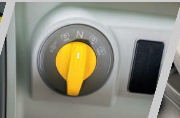
> Electrohydraulic PTO selection.
