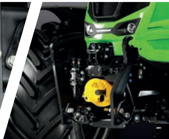
> 5450 kg lifting capacity and DualSpeed front PTO.
