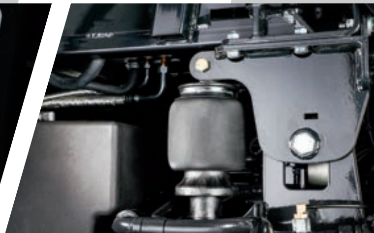
> Pneumatic cab suspension for a smoother ride.
